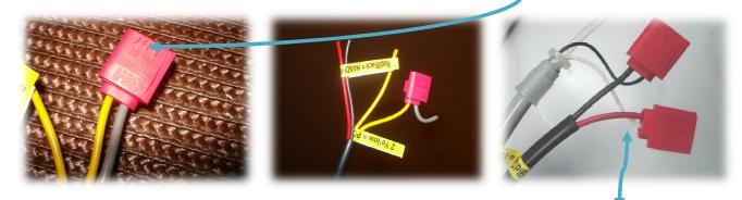
On the tray side repeat the same method for the handpiece and power control wires. **NOTE** the handpiece wires are *thinner and care should be noted* that the wires are fully inserted and align straight in the *metal clamp blades* to make a secure connection.
